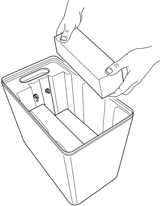
**THIS SOFTENER CAN ONLY USE BLOCK SALT. DO NOT USE TABLET, GRANULAR OR FINE SALT.**
